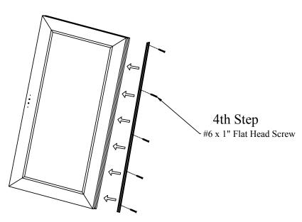
4th ~ Screw and Tape Interlock on to Operating Panel. (Multiple Places)
