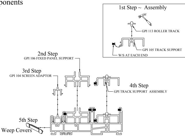
1st  $\sim$  Install Roller Track to Track Support. Along with 2  $\sim$  1" Weatherstrips at each end (as shown)
