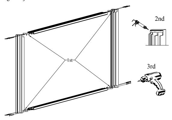
1st ~ Apply one Gasket on each end of the jamb at the sill and head.
